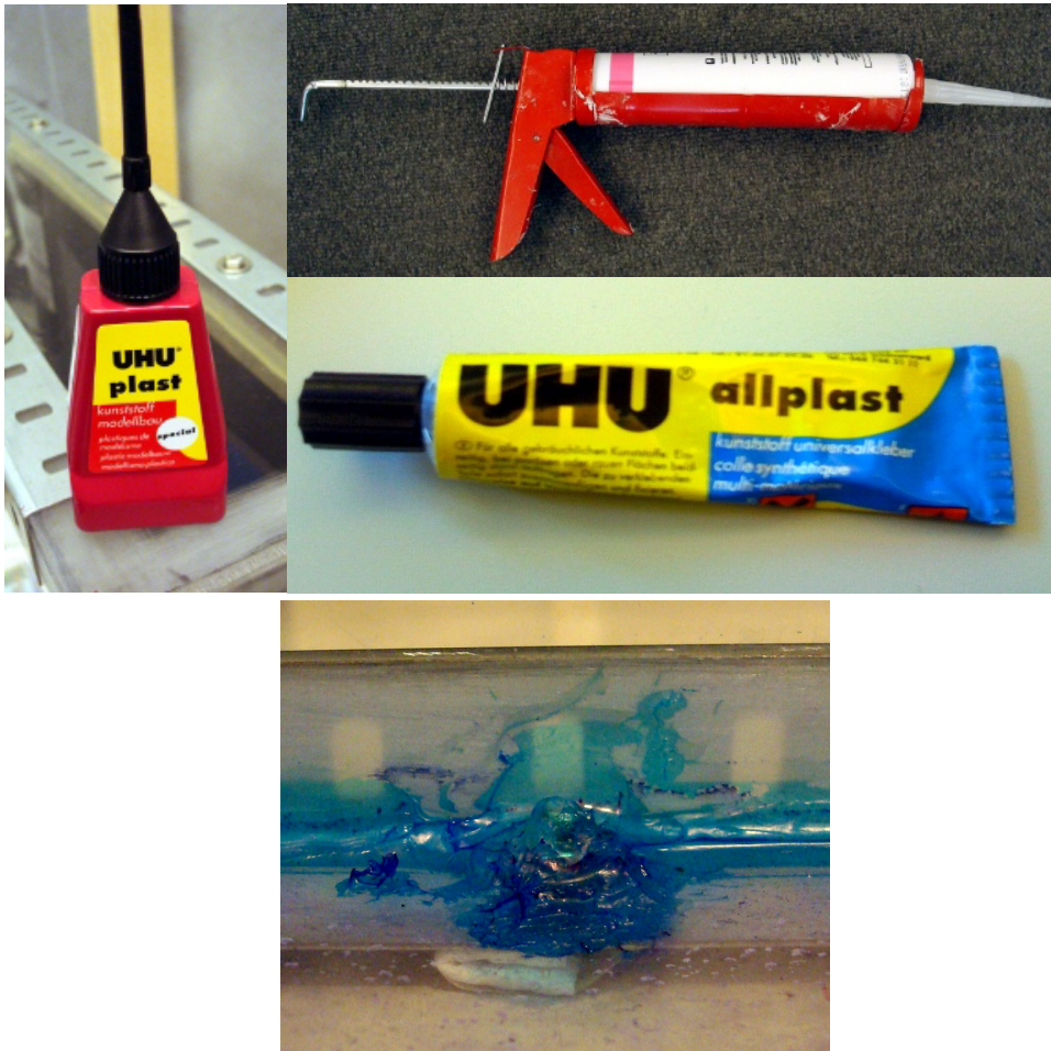
Figure 3.5.: The upper images show the three sealing products which were used. The lower picture shows how a screw needs to be covered by silicone in order to seal it. Originally, the silicone was transparent but as a result of the utilized colorant to dye the water it took on its color.
