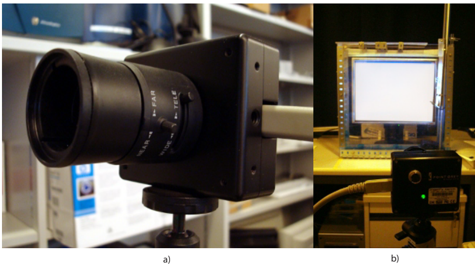
Figure 4.1.: Image a) shows the utilized Dragonfly Express and image b) depicts the setup including camera, tank, wedge and flat screen.
