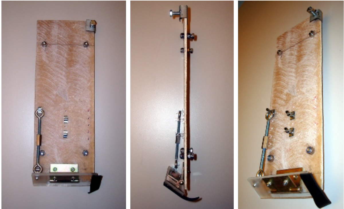
Figure 3.9.: The images above show different perspectives of the adjustable wedge that produces the splashes.
