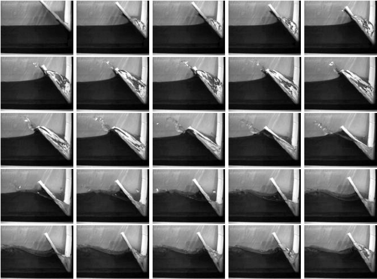
Figure 8.1.: A sequence of images which were taken from an experiment in a fish tank. The depicted pictures show every second image of the real data, effectively with 100 frames/second. Contrast adjustments were applied.
