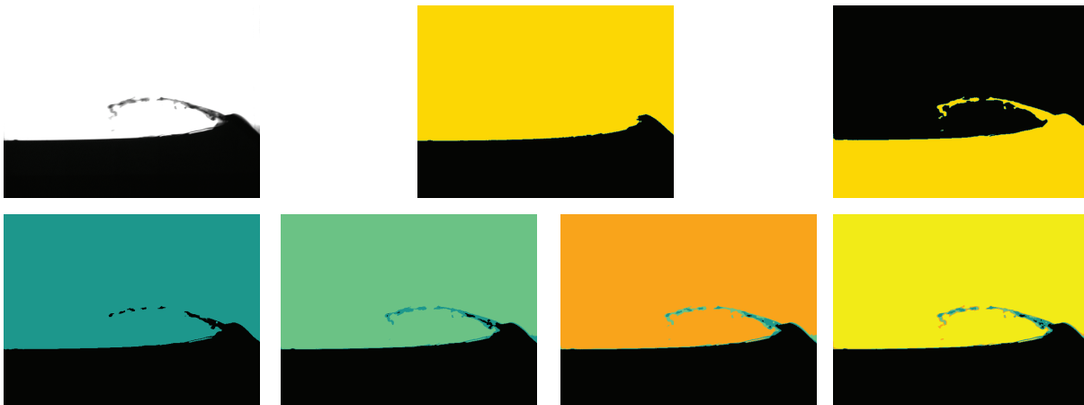
Figure 6.6.: The top left image is the original experimental image. The other images on top are segmentations with the region growing algorithm. Once with the seed point in the fluid (central image) and once in the background. The lower images are all segmented by k -means with 2, 3, 4 and 5 classes, from left to right accordingly. The results obtained with the graph cut algorithm are omitted since they do not show any observable difference from the k -means results.
