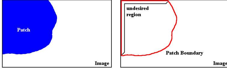
Figure 3.1: On the left side, a patch that is reaching over the image border is displayed. The region that the patch is representing is very likely to go beyond the image boundary. This leads to undesired positions in the patch boundary, which will lead to random feature information.
